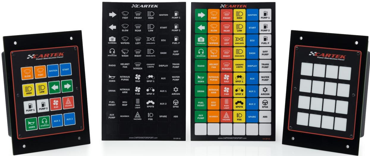
The CARTEK Power Distribution Panel is a fully integrated, fully electronic solution to power distribution in race and rally cars. Designed to replace 16 Fuses, Relays and Switches as well as a variety of control systems, these units therefore greatly simplify the wiring, reducing build time, saving weight and maximising reliability.
