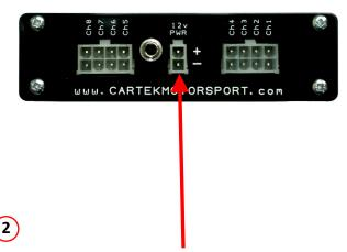
Whilst still holding both buttons connect power to the Relay Unit
