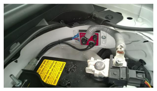
The Isolator should be mounted directly to the vehicle's metal chassis close to the vehicle's battery but away from any high temperature sources.
