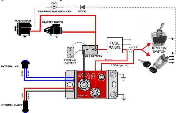
For cars not fitted with alternators it is not necessary to connect anything to the terminal marked FUEL or IGN as the battery disconnection will cause the engine to stop.
