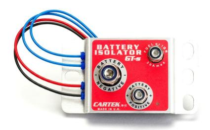
The **CARTEK** Battery Isolator GT is a fully electronic 'master/kill switch' system designed specifically for race car applications. This device contains no moving parts and the solid construction provides very high resistance to shock, vibration, water and dirt. Using the latest MOSFET technology this Battery Isolator provides safe, spark-free isolation of the vehicle's battery and engine electrics.
